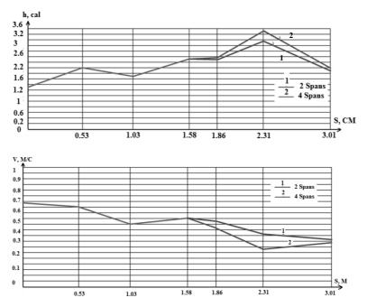
Fig. 3. Graphs of the level change concerning free surface of water and the flow velocity along the axis of flow on the area of its expansion
