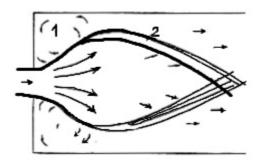
Fig. 1. Rapid flow spreading in wide channels: 1–whirlpool, 2–oblique hydraulics jumps
