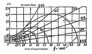
Fig. 2. The graph of current lines and the lines of equal depths
